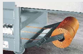
Convenient and firm strapping of the bales thanks to sophisticated strapping technology with polyester tape.
