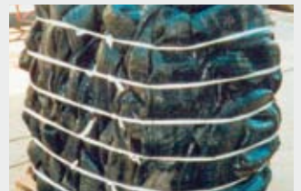
Optimum compression result with difficult materials, e.g. car tires on europallet.
